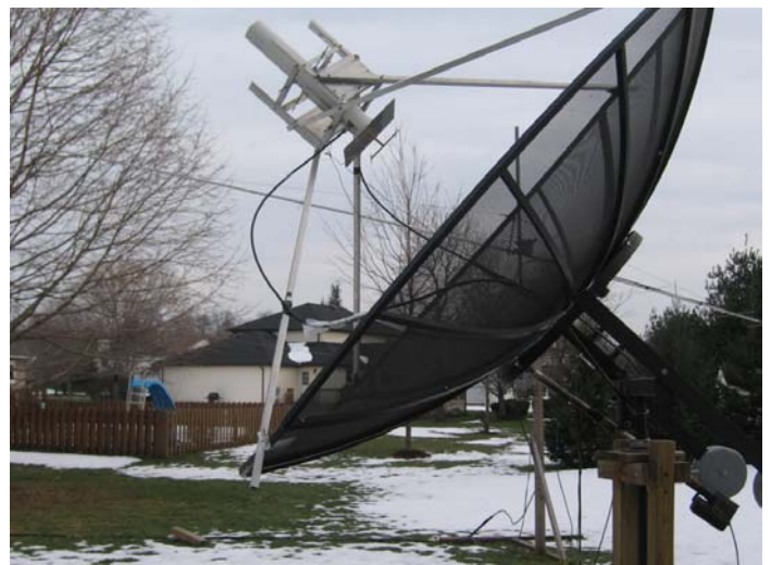
WA8RJF's dish used to make first 902 EME QSO with W5LUA in nearly 10 years. A dual dipole feed was used.
