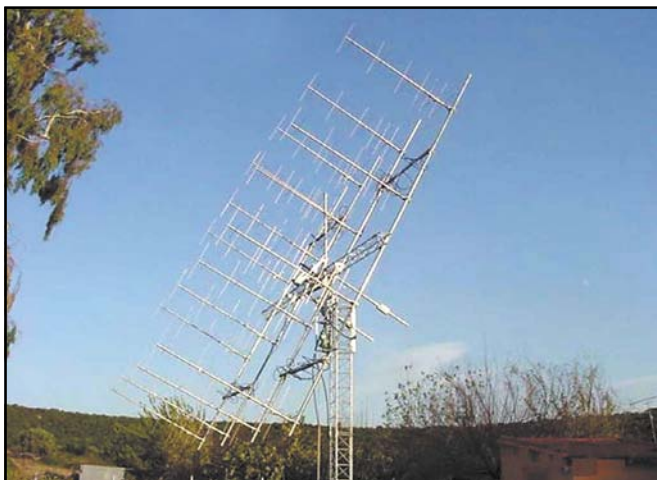
The 2-meter array (16×6 cross-polarized, 1.1 wavelength, 22 dBd) of Jimmie, SV1BTR.
