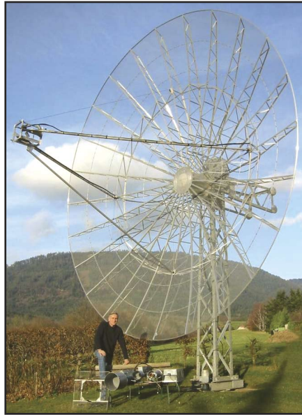
Longtime EME operator Philippe Pierrat, F2TU, with his homebrew dish and feeds for 432, 1296, 2304, 5760 and 10368 MHz.
