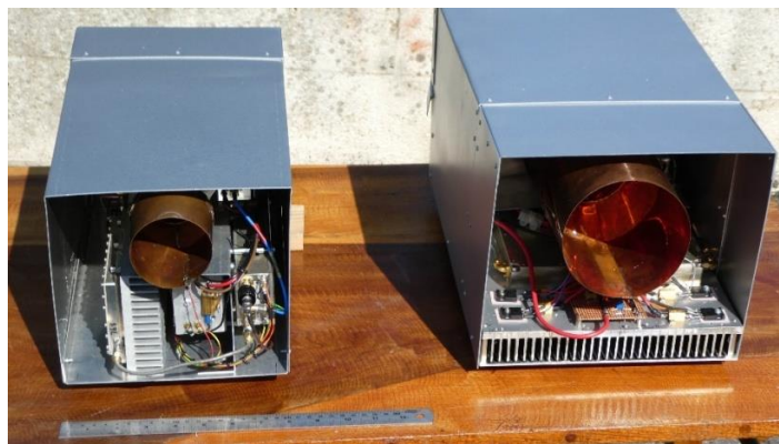
G4NNS' 6 cm feed box is on the left and 9 cm is on right with SSPAs
