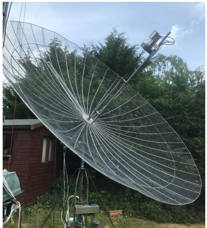
G4RGK's 4.5 m dish with 13 cm feed in place – getting ready for ARRL MW Contest
