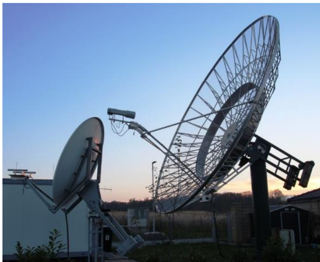
OK1DFC's dishes – 8 m offset dish (on right) use for 150 x 62 score in one WE!
