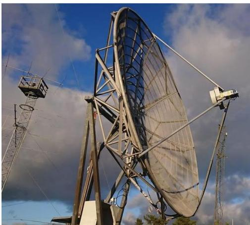
**SK0CT 6 m dish used in 23 cm SSB Funtest**
