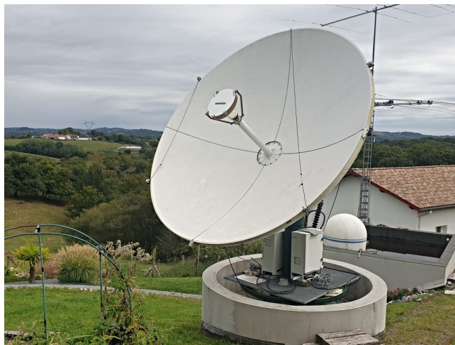
Parabola 3,7m F2CT na 10GHz s cassegrainem
